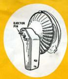
Occasionally a flashbulb may shatter when fired. To guard against this contingency, the diffusing screen must always be securely closed before using the equipment.
